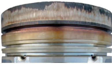
Special gas application after > 10,000 operating hours with GMO 240
